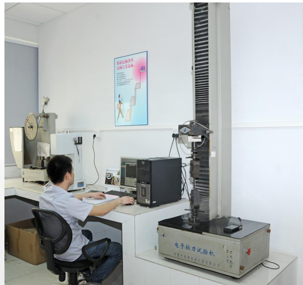
Universal Tensile Testing Machine (Tension, Bending, Elongation, Flexural Modulus)
